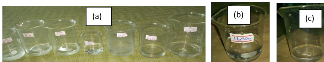
Figure 9. Solubility test of prepared bioplastic (a) initial test (b) and (c) after 1 hour
