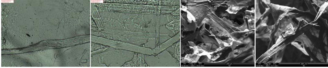
Figure 2. From left to right: optical microscope images (scale bars: 0.02 mm) of MFC-10 and MFC-15; and SEM images (scale bars: 200 \mu\text{m} ) of MFC-10 and MFC-15
